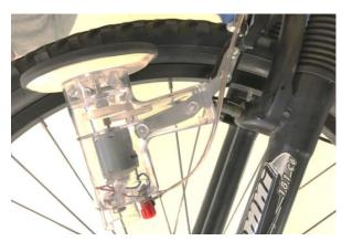
Figure 2a: RE-Brake attached to bike
