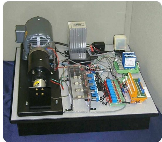
Figure 1. Motor Generator station
