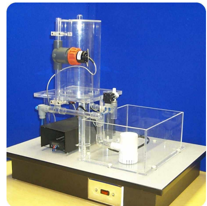
Figure 2. Variable speed pump-flow-level station
