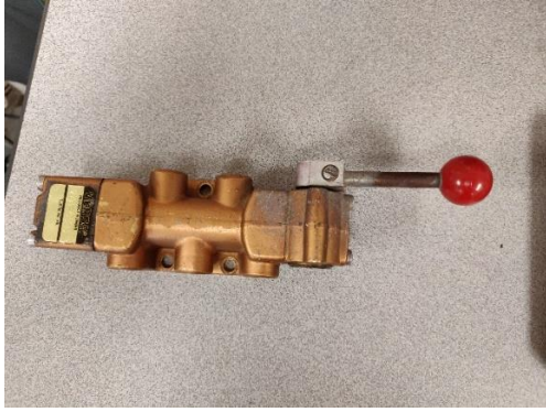
Figure 3. Original manual directional valve. Figure 4. New solenoid directional valve.
