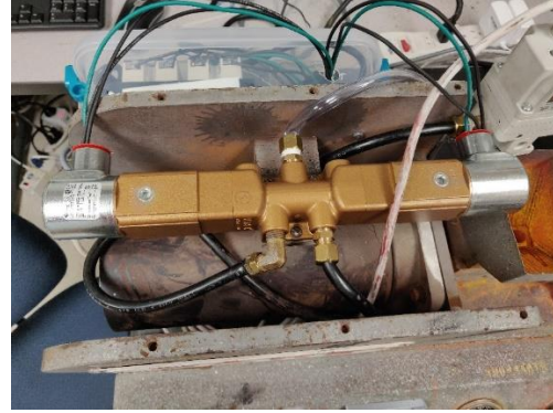
Figure 3. Original manual directional valve. Figure 4. New solenoid directional valve.
