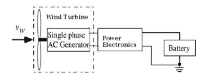
Figure 1: Physical Diagram of the Wind-Turbine-Battery System
