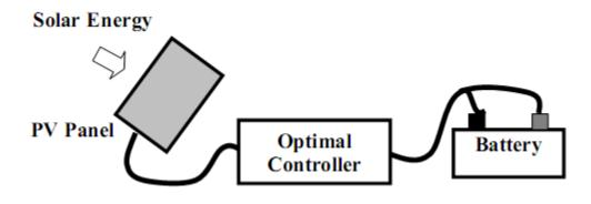
Figure 2: Schematic Diagram of a Solar Powered Battery Charger with Optimal Controller
