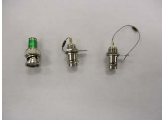
Figure 3. Load resistors used to determine parasitic inductance. Lead lengths are 0 mm, 15 mm and 60 mm.
