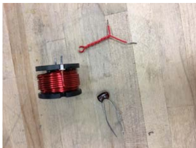
Figure 4. Iron core choke inductor with the “gimmick capacitor” and the a 300 pf capacitor.
