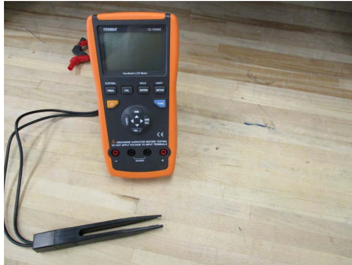
Figure A-1: Tenma Model 72-10465 LCR meter used to measure component values.
