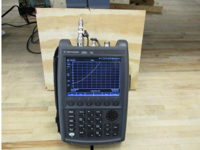
Figure A-3: Experimental setup used to determine parasitic reactance of a resistor using an RF analyzer that measures SWR.
