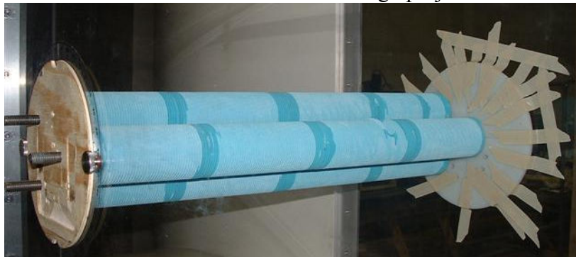
Array of cooling fins (.030" thick x 2.4" diameter X 24" long) in wind tunnel – Senior Design project
