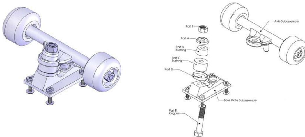
An example of a student project illustrating the dynamic geometry is seen in Fig. 4. Here, an avid skateboarder in choosing an object of considerable personal interest, also was able to gain some insight into some aspects of engineering and manufacturing and by doing so successfully completed the geometric modeling exercise.
