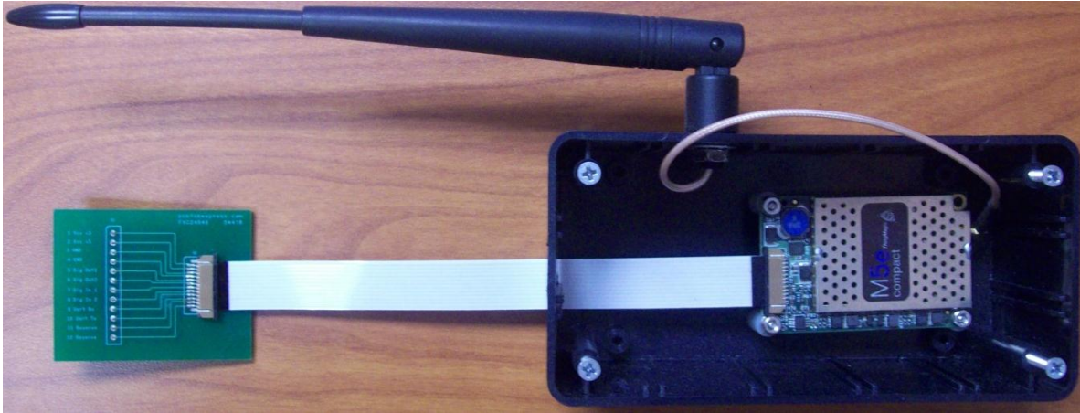
Figure 1. Enclosure Box, RFID Module, and PCB.
