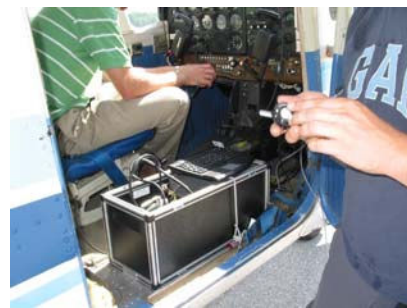
Figure 6b: Terrahawk System installed in Cessna 172
