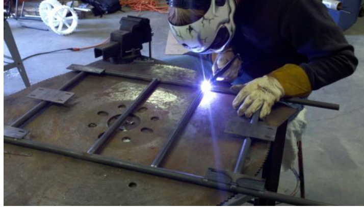
Figure 7: Welding the frame
