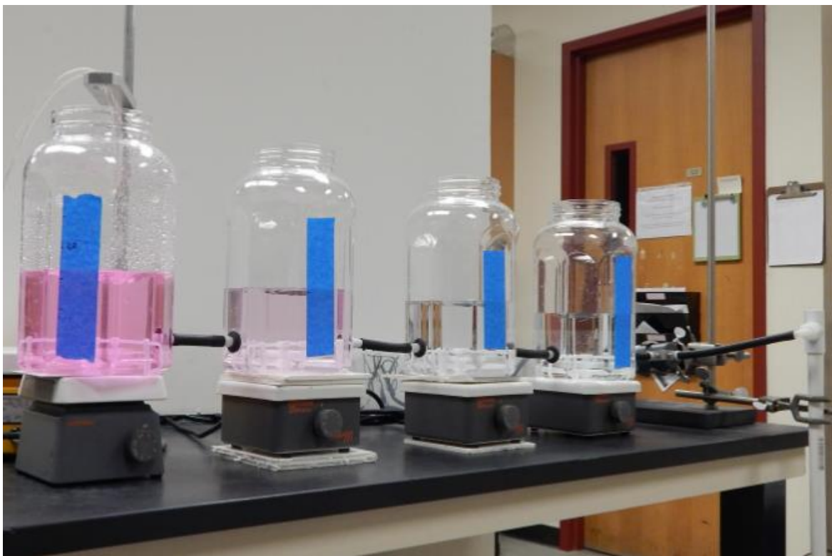
Figure 6. Sensor-based Dye Tracer Experiment with Four Mixed Reactors in Series.
