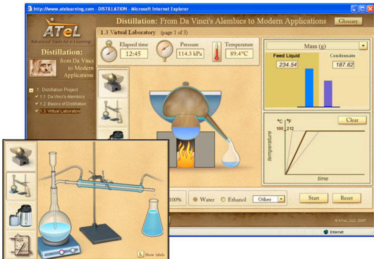
Figure 4. A set of virtual laboratories enables students to conduct experiments and collect virtual data. Students can choose a liquid from a list. Using the tool bar on the left they can select labware. They can also be able to vary the heating rate and observe the dynamics of the processes.
