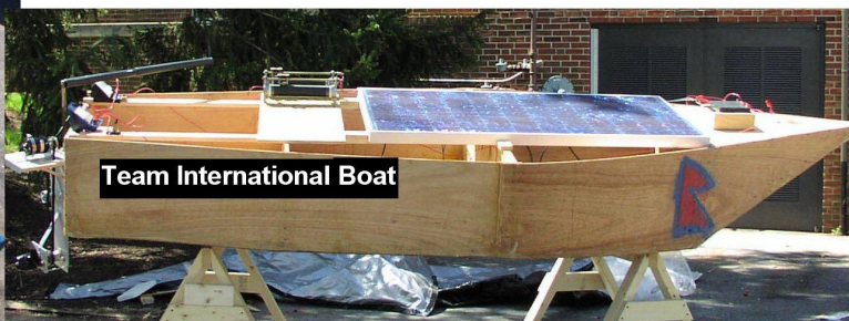
Figure 3: Final construction of solar boats capable of carrying one person. Construction was by teams of 7 - 8 first-year engineering students. Prefabricated boats or trolling motors were not allowed for the project.
