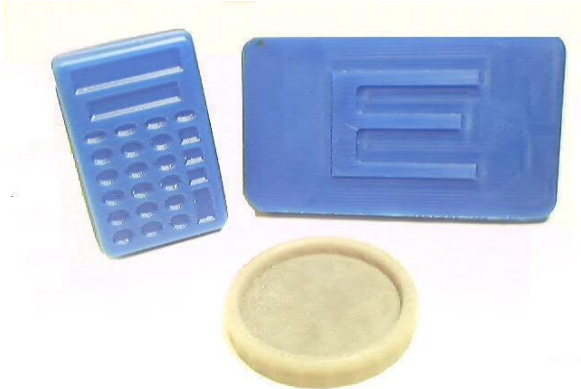
Figure 1 Solid Modeled and CNC Mill Manufactured Wax Parts
