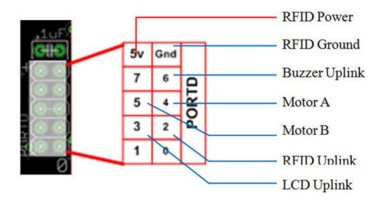
As shown, the RFID runs off the power and ground, with its uplink to the PCB in PD.2. The LCD Uplink is wired into PD.3. The Motors run off PD.4 and PD.5 for uplinks. The buzzer uplinks to PD.6. Power and ground for everything besides the RFID are run off the board itself, not PORTD.
