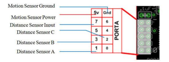
As seen here, each pin has a specific use. The three distance sensors and the motion sensor run off of PORTA. Though it's configured to be a PIN actually, and receive inputs from each sensor.
