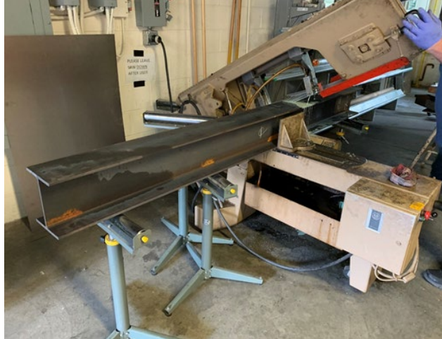
Figure 2: The process of cutting steel pieces to desired sizes
