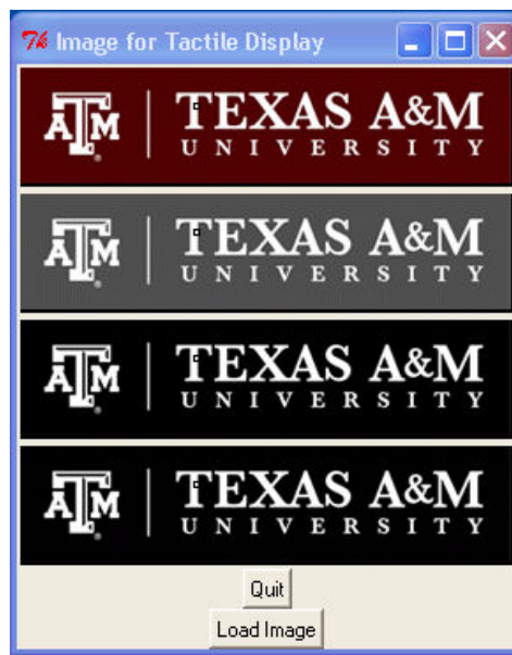
Fig. 4. Graphic User Interface showing four copies (full color, red portion, blue portion, green portion, respectively) of a digital image. The small square box (on the “T” of “Texas”) indicates which pixels are currently being used to move the display pins.
