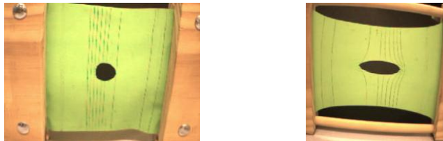
Figure 3 Latex Sheet with a Hole in Tension showing the stress flow lines
