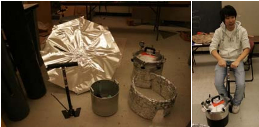
Figure 4: (left) The sterilization prototype, consisting of a non-electric autoclave, high pressure pump, and equipment to allow solar heating of the autoclave and (right) a team member putting the autoclave through a drying cycle through manual pumping.
