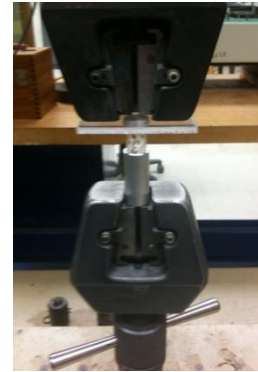
Figure 7: Universal test machine during compression test with acrylic sheet.
