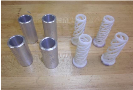
Figure 6: aluminum sleeves and 3D printed fastener
