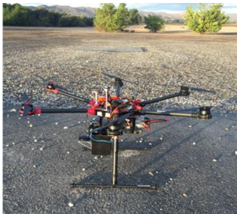
Figure 11. DJI S900 Hexacopter Equipped with a LIDAR.
