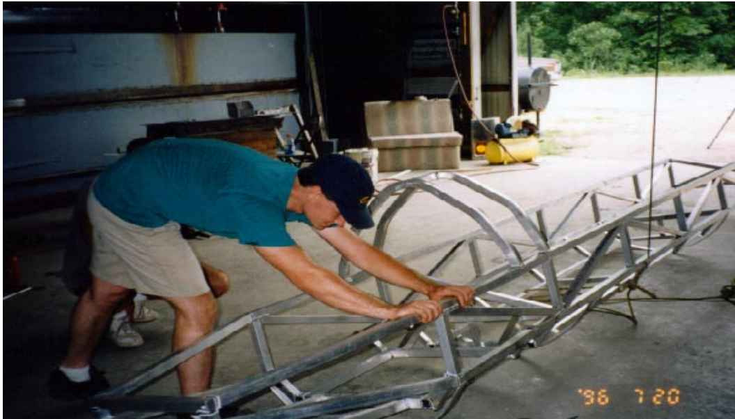
FIG 1. Aluminum main frame and built-in double roll cage for MTSU's solar car, the Solarraider II.
