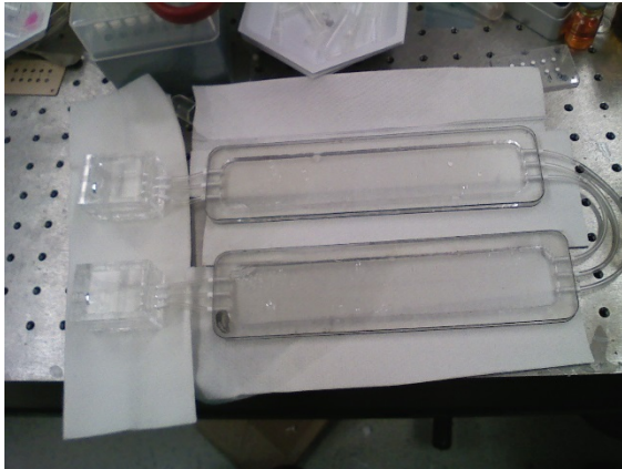
Figure 3: Constructing the Algae Bioreactor system. From [2].
