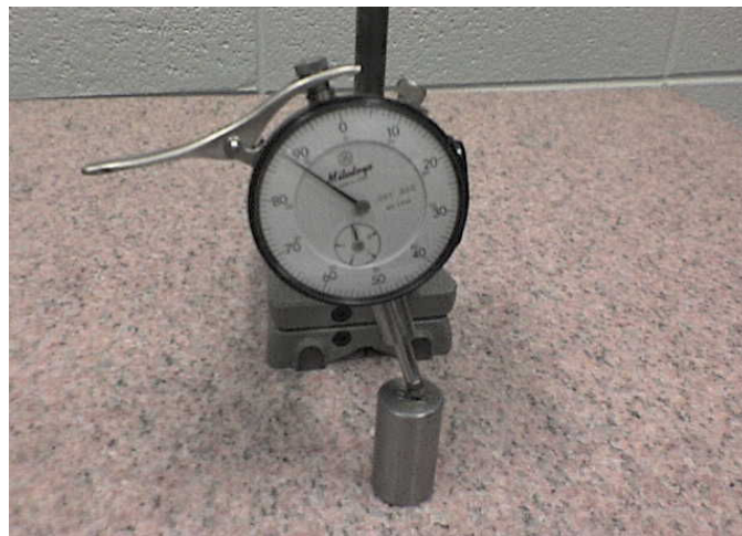
Figure 4. The concept of cosine error.
