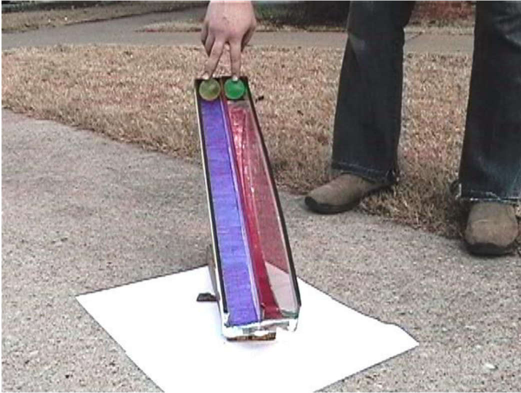
Figure 6. The cycloidal and straight path model built by one ET 1840 student team.
