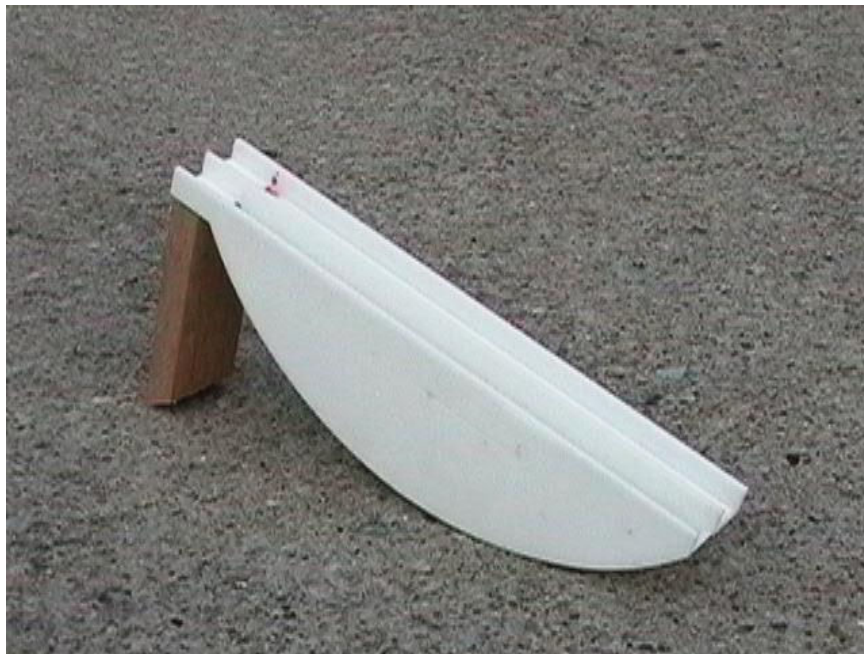
Figure 2. Prototype of the cycloidal and straight path model built on the Stratasys machine.
