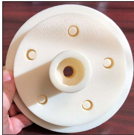
Figure 8. 'Bad' part passes inspection when datum priority not followed.
