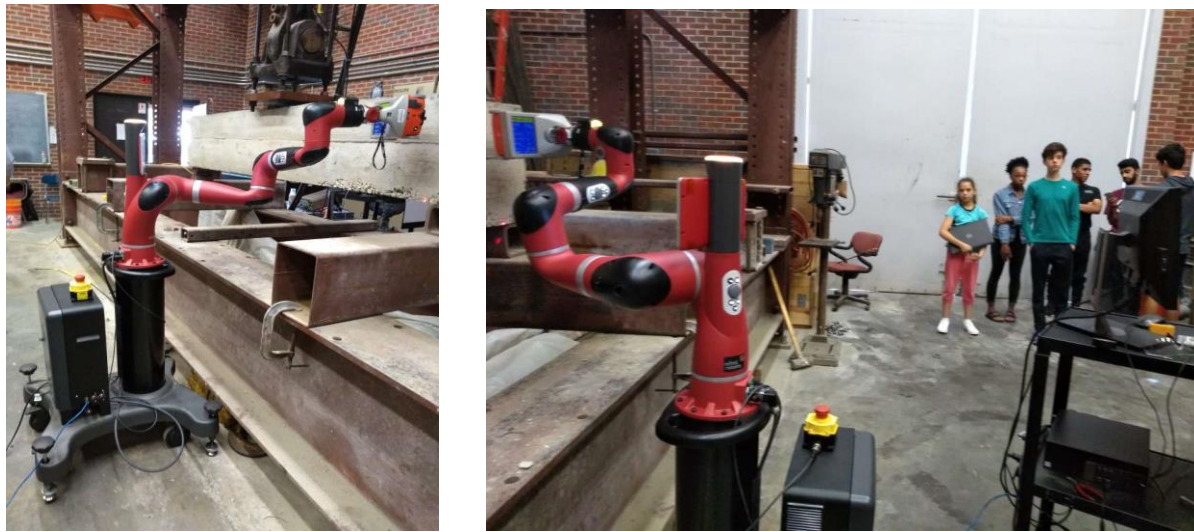
Figure 11: NDT (non-destructive Testing) Robot to scan the concrete surface.
