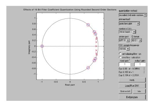
Figure 6. Pole-zero plot of 7th order IIR Elliptic digital filter, quantized to 16 bits and implemented as a Direct Form II transpose using fixed-point algorithms.
