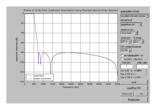
Figure 5. Magnitude plot of 7th order IIR Elliptic digital filter, quantized to 16 bits and implemented as a Direct Form II transpose using fixed-point algorithms.
