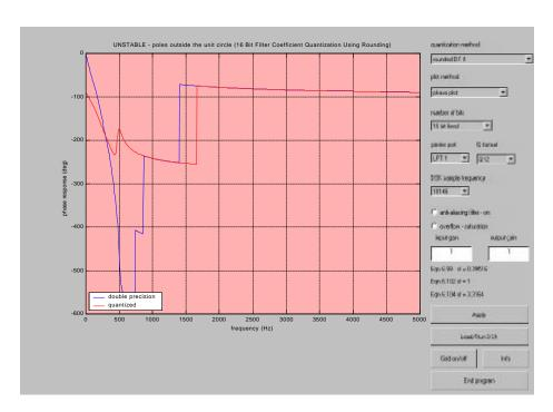
Figure 3. Phase plot of 7th order IIR Elliptic digital filter, quantized to 16 bits and implemented as a Direct Form II transpose using fixed-point algorithms.
