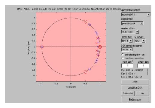
Figure 4. Pole-zero plot of 7th order IIR Elliptic digital filter, quantized to 16 bits and implemented as a Direct Form II transpose using fixed-point algorithms.
