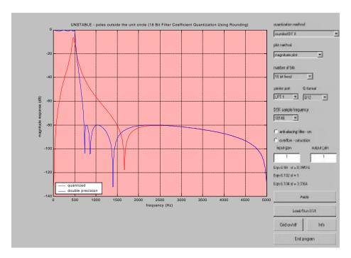
Figure 2. Magnitude plot of 7th order IIR Elliptic digital filter, quantized to 16 bits and implemented as a Direct Form II transpose using fixed-point algorithms.
