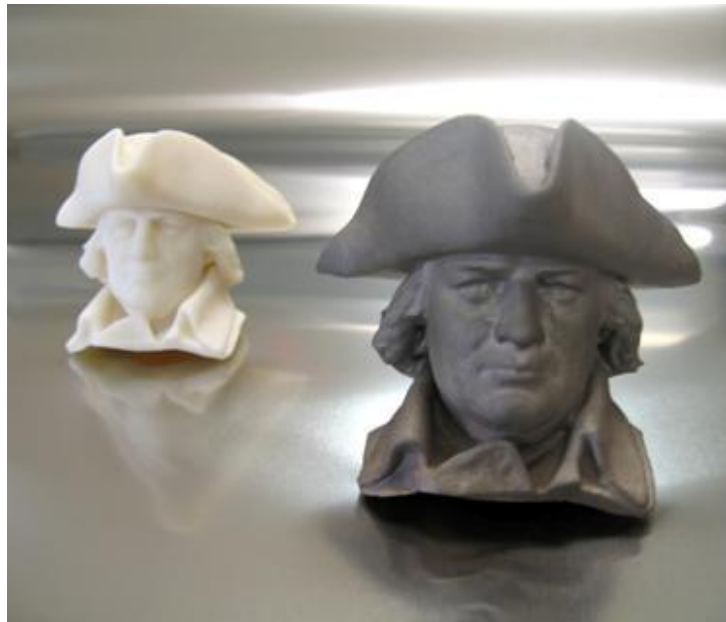
Figure 3. Rapid prototyped replicas of the original piece (Fused Deposition Modeling – left, 3D printing – right)
