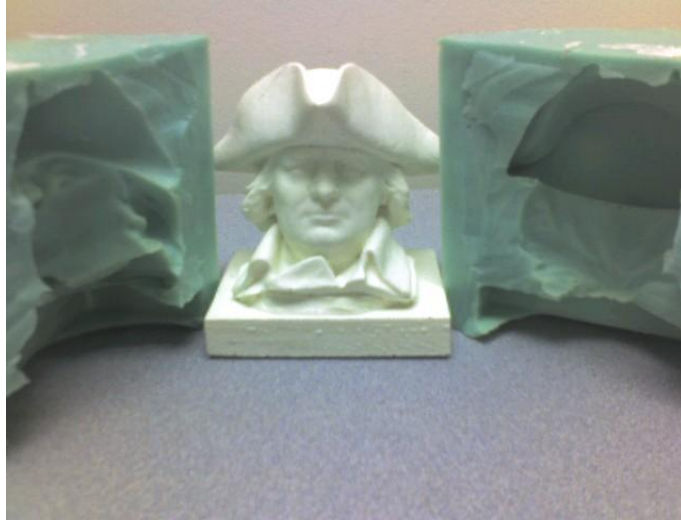
Figure 4. RTV molds halves and a polyurethane copy made by them
