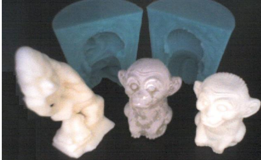
Figure 6. A rapid prototyped replica (left/front row), silicon rubber mold halves (back row) and their pattern (middle/back row), and the resulting polyurethane replica (right/front row)
