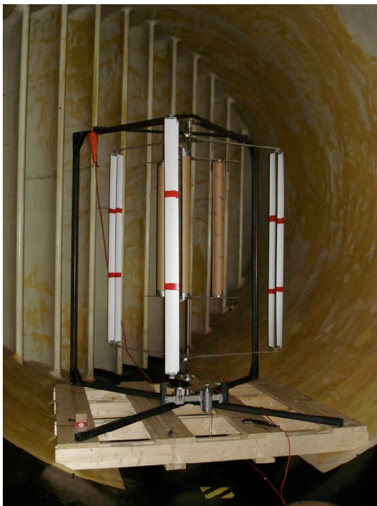
Figure 2: 2m Wind turbine with flexible blades in wind tunnel testing
