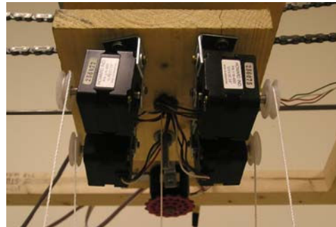
Figure 4 Pulley and stepper motor assembly
