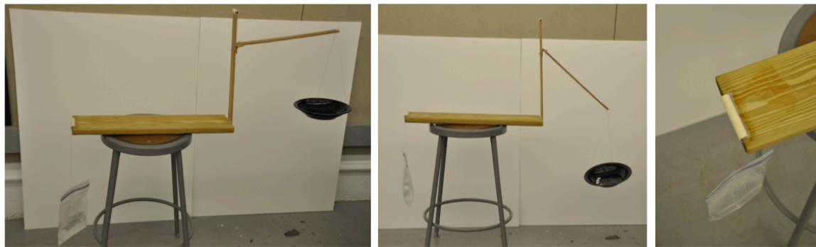
Figure 8: Device with multiple states of equilibrium. Plastic piping and fishing line used to approximate a frictionless pulley
