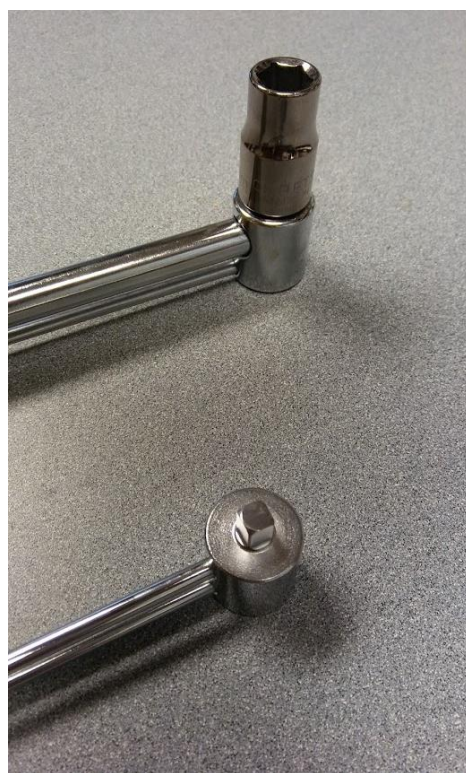
Figure 4c Torque wrenches (the top one has a hex head socket 1/2" drive adaptor while the bottom one needs a 1/4" drive socket adaptor)
