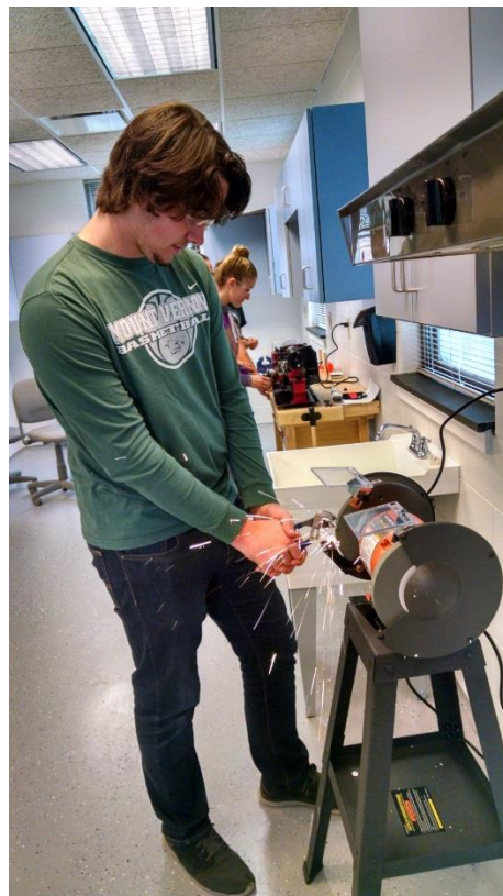
Figure 3 Grinding flat surfaces on the bolt body
