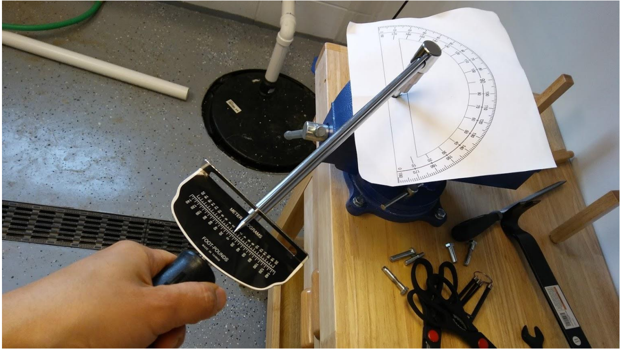
Figure 6 Applying torque through the torque wrench handle
