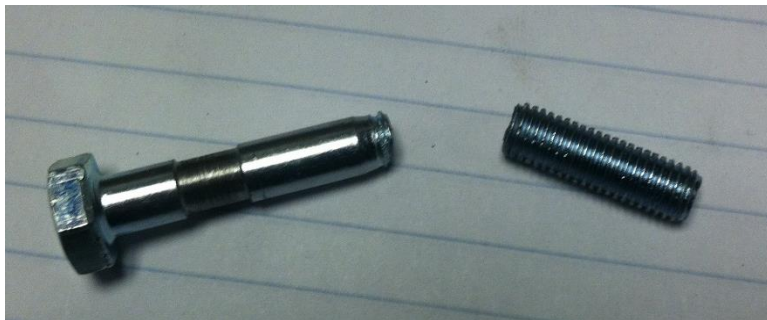
Figure 10 Bolt broken at the threaded area
