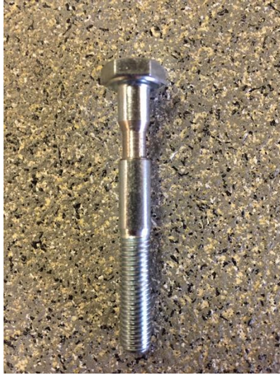
Figure 2 Bolt after neck being turned down
