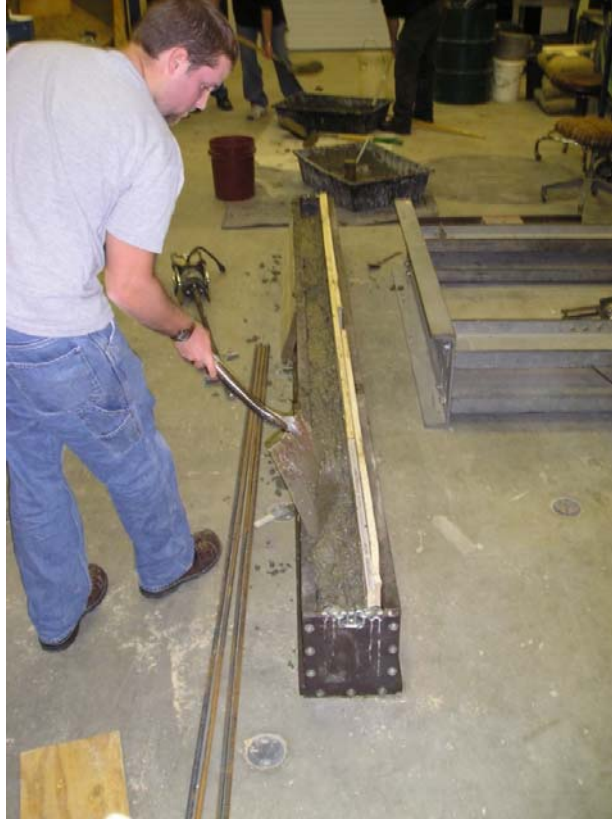
Figure 1 Casting the beam.
