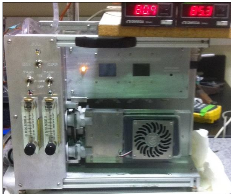
Figure 1. Front view of the Desktop Learning Module (DLM) with an extended area heat exchanger cartridge.
