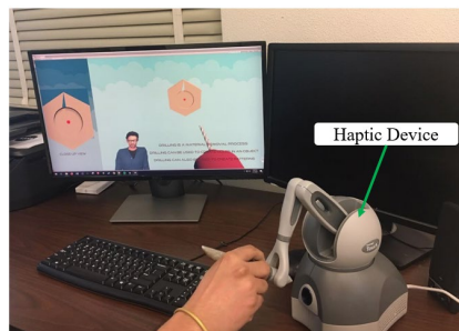
Fig. 4. A student interacting with a non-immersive haptic based VLE to learn drilling concepts.
