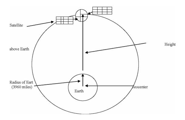
The above sketch shows the height of the satellite from the center of the earth. For example: If a satellite is 7500 miles above the earth in circular orbit it simply means that, the distance from earth to the satellite location is (3960 + 7500) miles since the radius of earth is 3960 miles.
