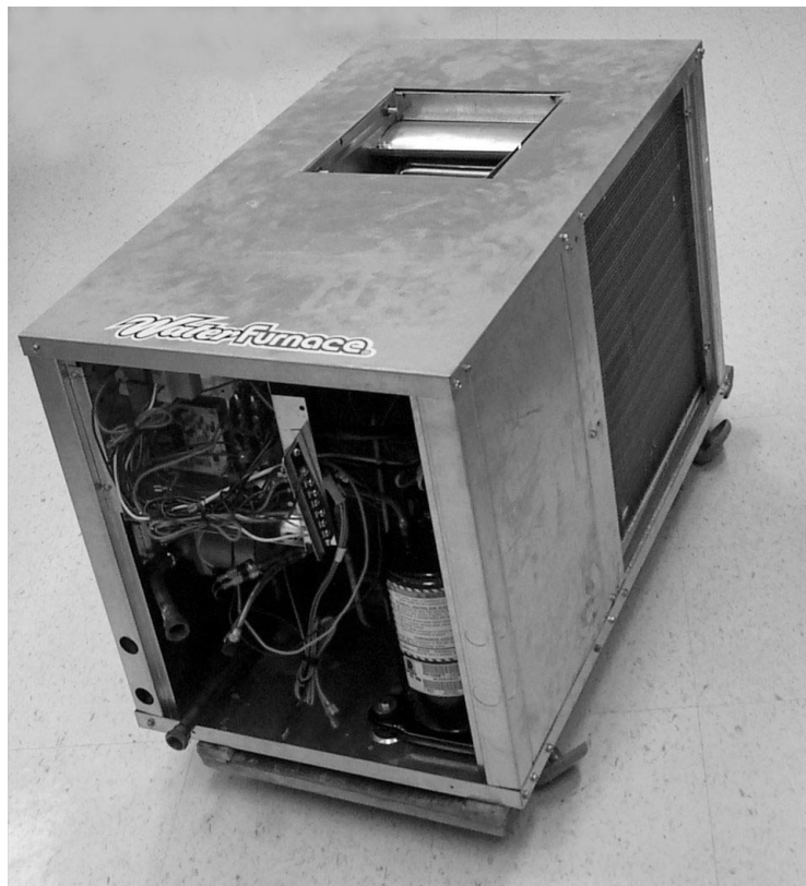
Figure 3: Heat Pump Water Heater
