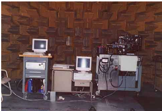
Figure 2 Portable small engine dynamometer
