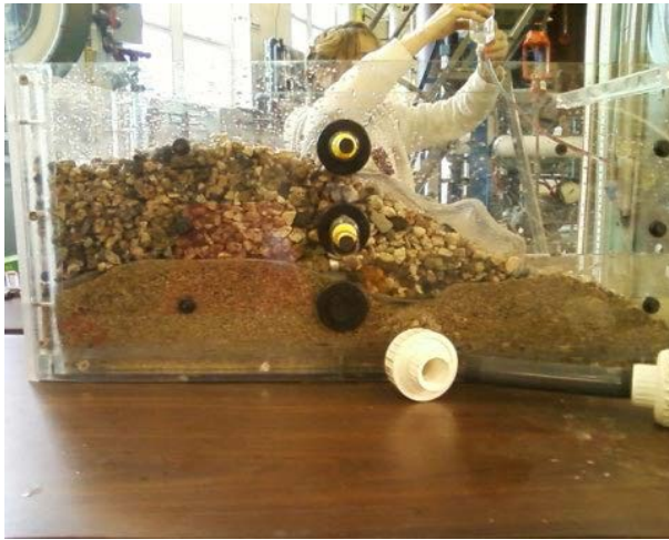
Figure 5. Image of a group's model river, filled with sand and rocks, prior to filling with water. The height of the sand and rocks in the image is similar to the topographic depiction of the island in Figure 4. Flow would likely be from left-to-right in the river bed, with water introduced through a port on the side of the plastic frame.
