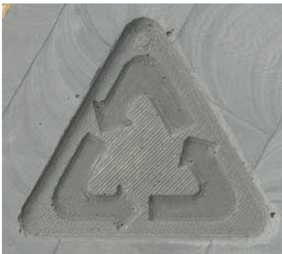
Figure 3: Surface of mold created by casting epoxy over unfinished RP model.
