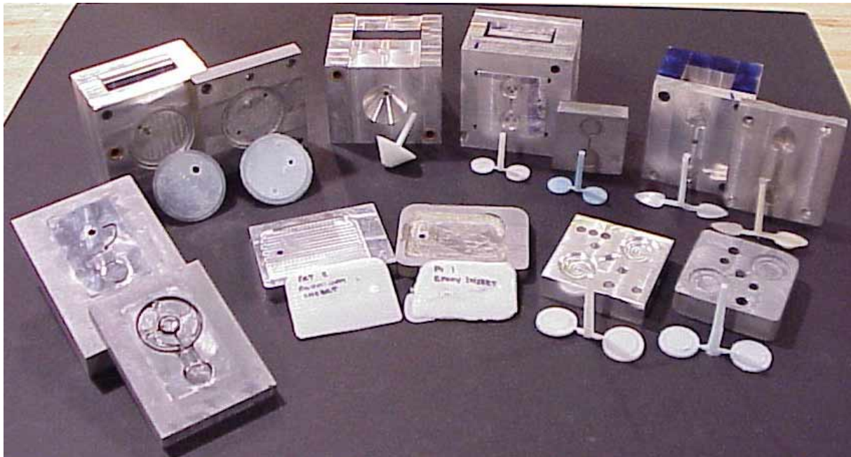
Figure 6: Seven mold sets manufactured using traditional machining and prototype construction methods.
