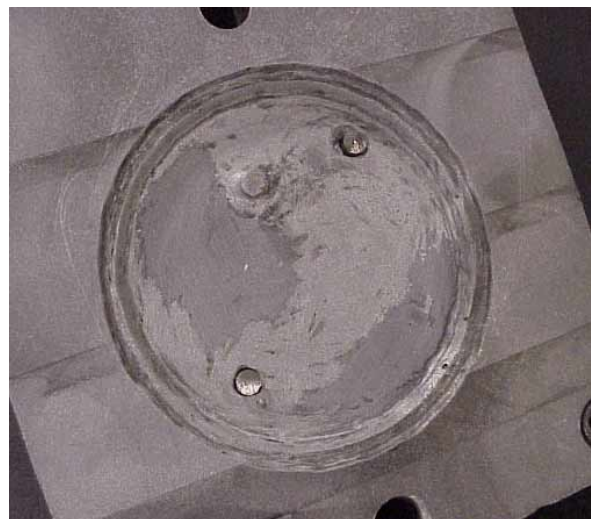
Figure 4: Patched and sanded mold surface to correct voids caused by primer.
