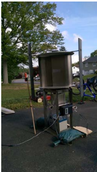
Figure 8 Prototype of the Integrated Wind and Solar Kit
