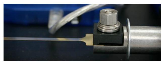
The black anodized aluminum grip has a rounded edge along the left edge, which clamps the brass strip against the stainless steel puller. There is a single-point contact at the right, and the stud passes through the center hole of the grip. Spherical washers ensure good clamping by the nut regardless of the specimen thickness.
