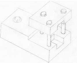
sample size. A single wing nut holds the shell in each clamp jaw, eliminating the need for tools (but requiring small fingers?) The entire fixture is gripped by the existing clamps, however wing nuts replace the existing hex nuts.
