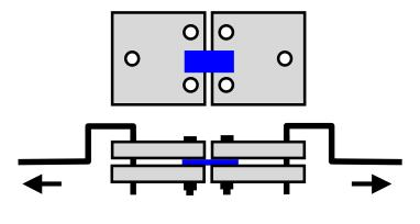
and nuts. Hooks passing through holes were connected to the tensile testing machine.
