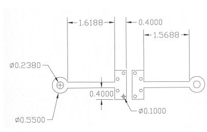
about an inch and a half out. For that side it seems that the best side of the piece is the longer of the two. After you have figured this part out one can notice the 4 holes on each end of the two pieces. These holes are to be threaded with a bolt of the department's choice. I chose to do it this way rather
