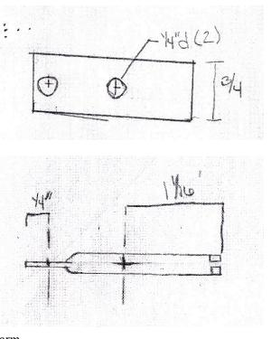
The clamp will attach to the PASCO tester in the same manner as the supplied specimens that come with the machine. This style will allow the user to adjust the pressure applied in holding the specimen by simply turning a screw.
