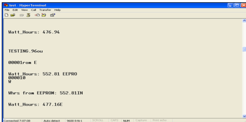
Figure 3: Screen capture of program acquiring watt-hour readings
