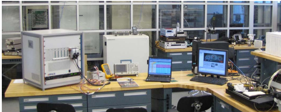
MSU's hardware-in-the-loop test bench composed of dSPACE donated components
