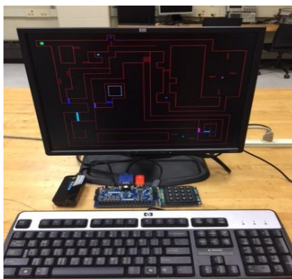
Fig. 1a video game system with Xilinx Artix-7 FPGA, Basys-3 Educational Board
