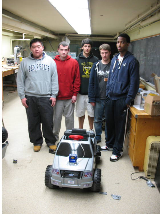
Figure 3. Front view of vehicle showing position sensor mounted on hood.
