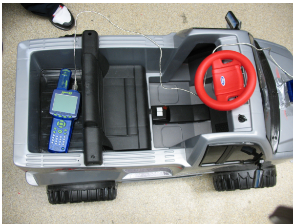
Figure 2. Top view of vehicle showing data logger in rear and speed sensor on hood
