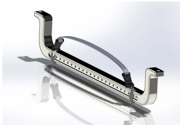
Figure 3 Front axle assembly from an early Ford
