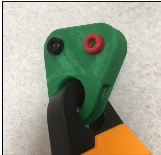
Figure 6. Closed Completed Assembly on Current Probe
