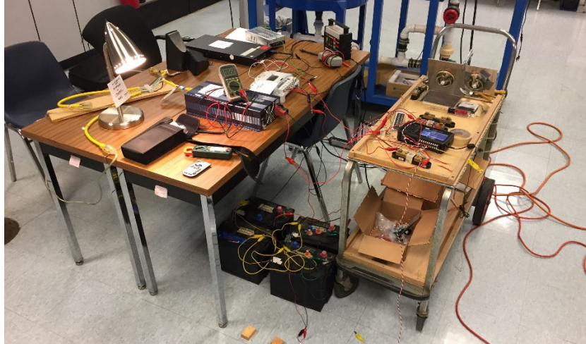
Figure 8: This shows the actual bench test simulation setup configuration in the lab to simulate PV module input. An incandescent lamp is used in this configuration as an AC load downstream from the inverter. To address safety concerns only authorized lab staff were allowed into the lab during these bench tests.
