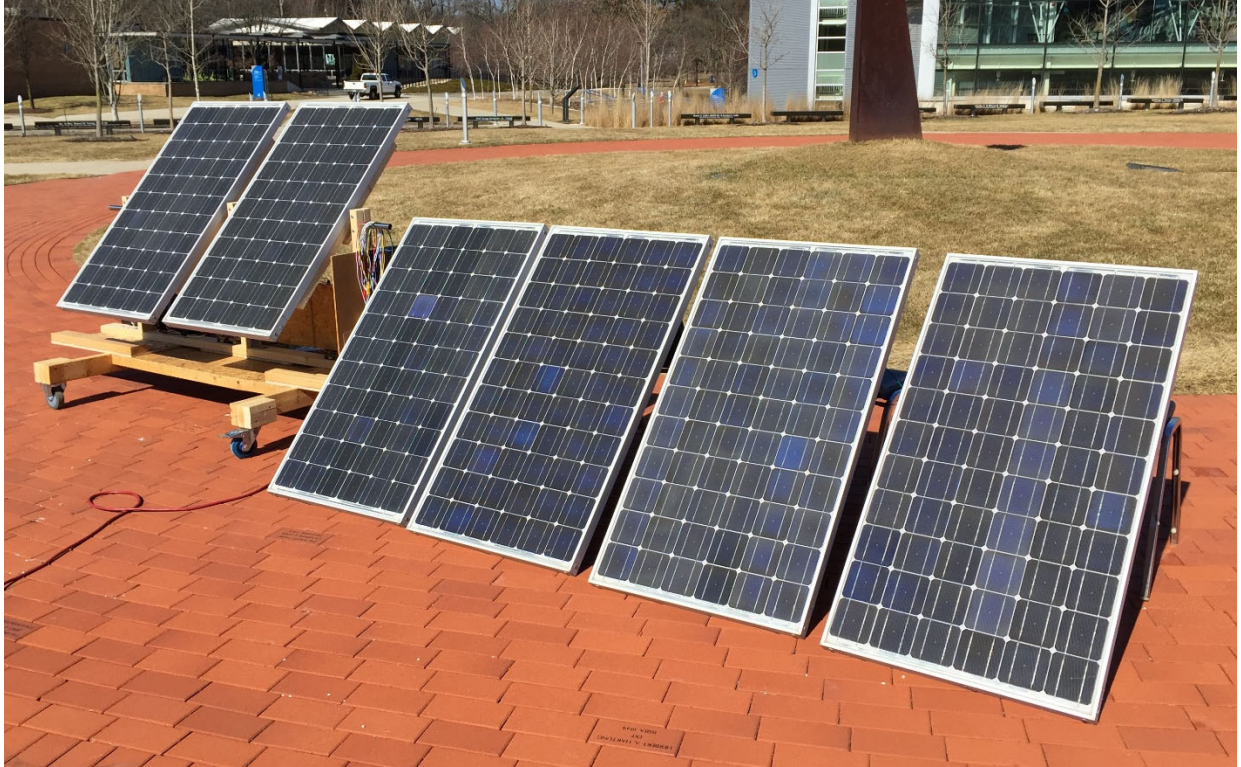
Figure 16: The six module system using the two modules mounted on the base cart with additional power input from the four stowed modules (the four modules to the right of the cart), for a total of six PV modules providing power with three sets of modules in parallel with two modules in series in each parallel set. Circuit connections for the set-up shown here were made using temporary jumper cables for the four modules that will be stowed on the cart.
